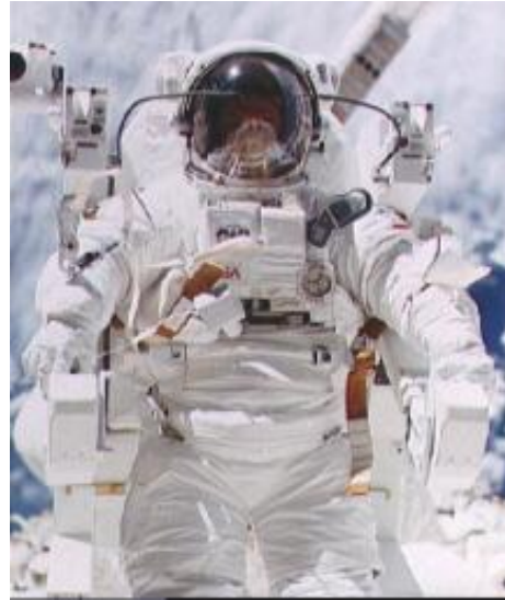
EMU Hard Upper Torso and Helmet with Display Module on Chest
